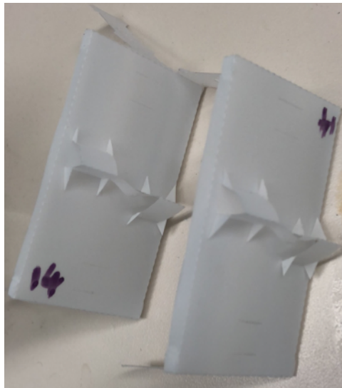
Figure 8: Two fabricated mechanical logic. When fabricating, the key is to check for the bistability of the beam along every step of the beam. We make sure that the bistable beam is not folded or damaged in any way. Any change to the bistable beam that reduces its bistability will result in a complete redo of the fabrication process.
